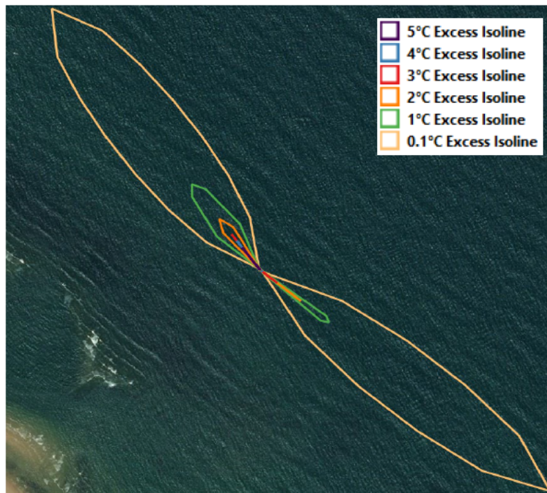
Figure 11. Zoomed extent of the CORMIX excess temperature isolines (°C) under mean spring, peak flood (SE) and ebb (NW) tidal states
